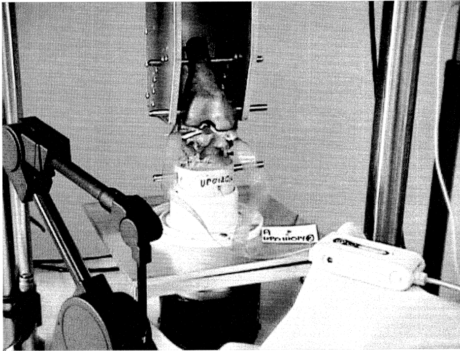
Figure 2 – Overview of experimental setup. A human cadaveric knee specimen was mounted in an MTS servohydraulic test machine with a fixed flexion angle of 30^\circ . An axial load of 1000 N was applied to the specimen, and intraarticular contact force, pressure, and area were measured in the medial and lateral compartments using a Tekscan K-Scan sensor. A Microscribe 3DX digitizer was used to record the location of three titanium bone screws mounted in the tibia and femur at the final static pose.
