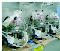
Fig. 1 Overview of the process used to evaluate computational damage predictions for a total knee replacement. (a) A constant wear factor is obtained from pin-on-plate experiments using the same material pair as in the implant. (b) This wear factor is used in a computational damage prediction that combines a dynamic contact model of the implant in an AMTI simulator machine with a surface evolution model. (c) The computational damage predictions are compared to experimental damage measurements made on the same implant during testing in a physical AMTI simulator machine.
